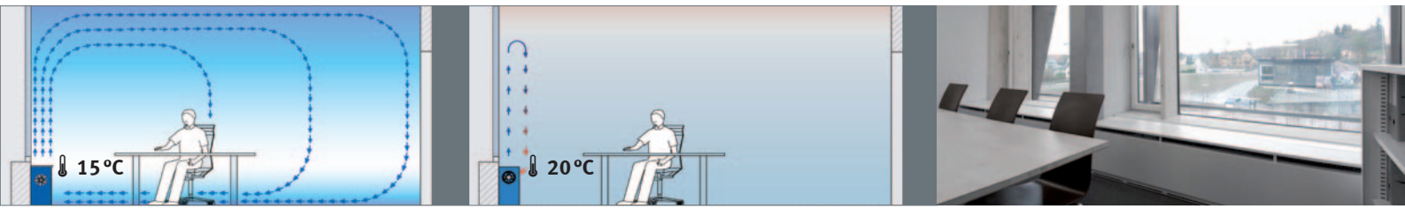
Conventional façade-mounted air-conditioning unit
